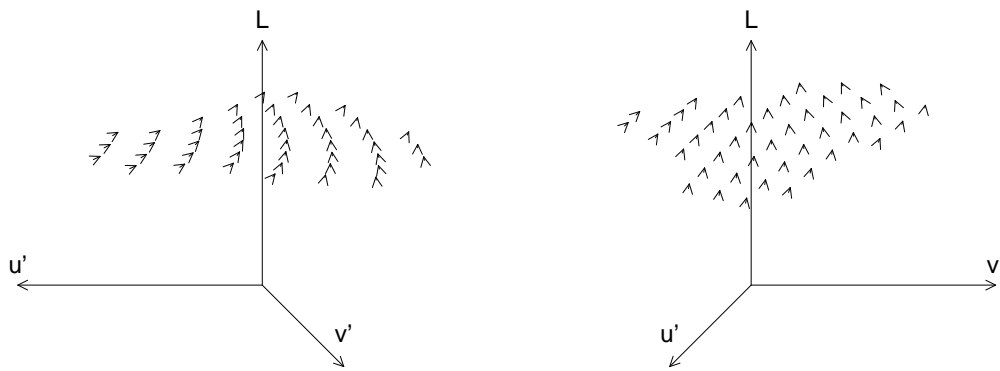
Figure 4.2: Two views of CIE (L^*, u^*, v^*) shifts for OSA plane L = 0 when the OSA PlaneSight calibration with \gamma = 2.3 is applied to a monitor with \gamma = 2.2 .
