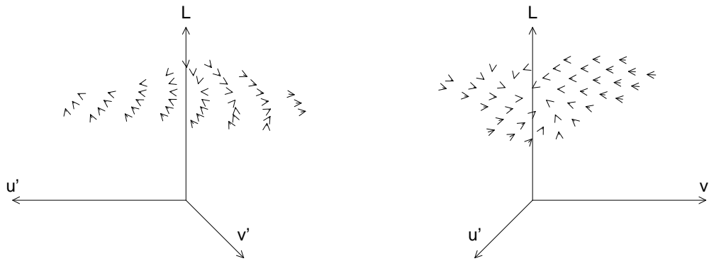
Figure 4.14: Two views of CIE (L^*, u^*, v^*) shifts for OSA plane L = 0 when the OSA PlaneSight calibration is applied to a monitor with Conrac phosphors.
